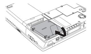
Figure 8-18 Installing the HDD pack
